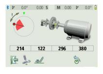
Rotate the shafts to the next position. The shafts must be rotated over a minimum of 45°.
