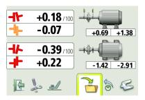
The Measurement Result screen shows coupling values and foot values in both the vertical and horizontal direction.
