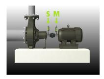
After rotating the shafts into different measuring positions, the system calculates the relative distance between the two shafts in two planes. The distances between the two measuring planes, distance to the coupling and distances to the machine feet are entered into the system. The display box then shows the actual alignment condition together with the position of the feet. Adjustment of the machine can be made directly, according to the displayed values.
