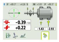
Rotate the shafts to the 3 or 9 o'clock position to make adjustments in the horizontal direction. The angle guide helps you to reach the right position.
