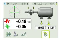
Rotate the shafts to the 12 or 6 o'clock position to make adjustments in the vertical direction. The angle guide helps you to reach the right position.
