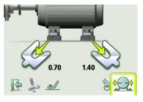
The Shimming screen shows foot values in the vertical direction as suitable shim values.
