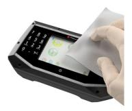
For the best possible function, the laser diode apertures, detector surfaces and connector terminals should be kept free from grease or dirt. The display unit should be kept clean, and the screen surface protected from scratches.
