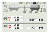
The screen displays measurement results, dimensions, target values if any, file name, date and time, serial number of the display unit, program, program version, calibration date and tolerances.
